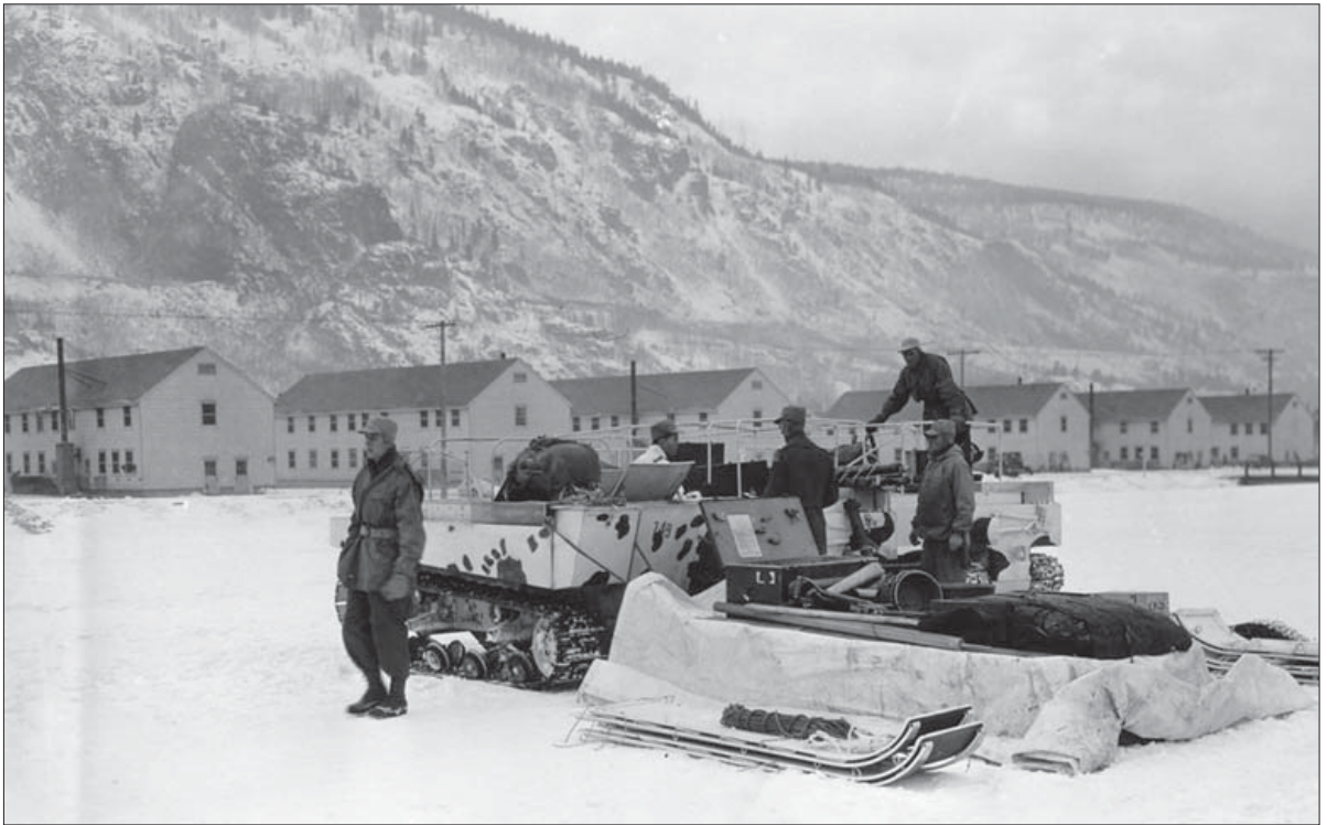
At Camp Hale, T15 (M28) Weasel cargo carriers – note the four angled bogie wheels – and a large towed sled being loaded with gear. On either side of the sled – its runners hidden here by a white tarp – are toboggans, which were towed by a skier. (Tom Laemlein/Armor Plate Press)
